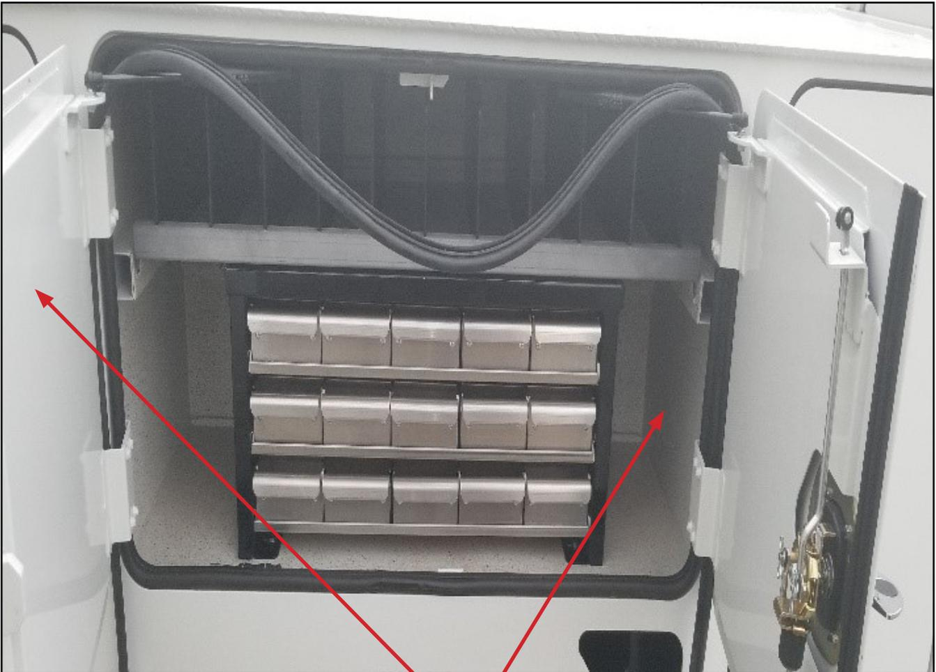
**POSITION THE DOOR GASKET IN THE CORRECT DIRECTION AND PLACE THRU THE HINGES FOR EASIER ADJUSTMENT AND INSTALLATION.**
