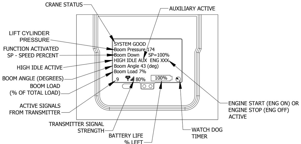
**CRANE STATUS**—shows current status of the crane. If any alarms are occurring they will be displayed here. Otherwise, it will say system good. **Note: Reference Troubleshooting section for alarm descriptions.**
