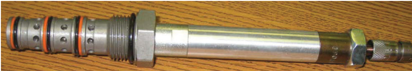
Verify movement in ports while manually overriding cartridge
