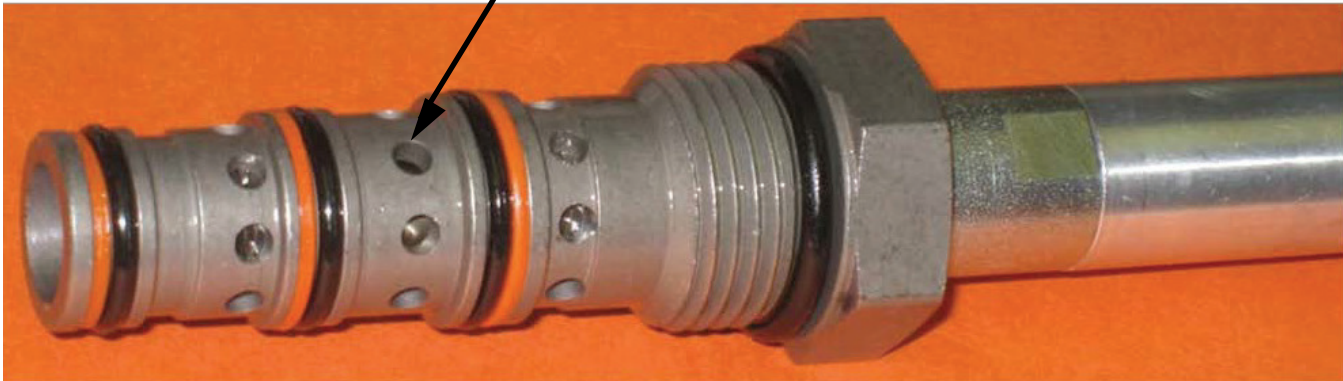
Verify movement in ports while manually overriding cartridge
