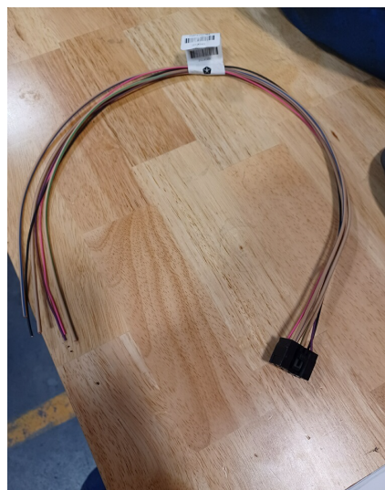
Figure 13 - "D" Upfitter Connector Location & Upfitter Harness
