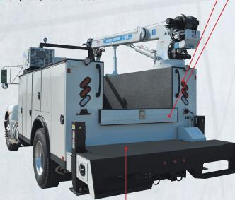
Over-sized workbench bumper with integrated step
