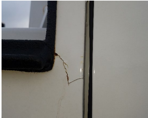
Figure 1 – Sheet Metal Crack
